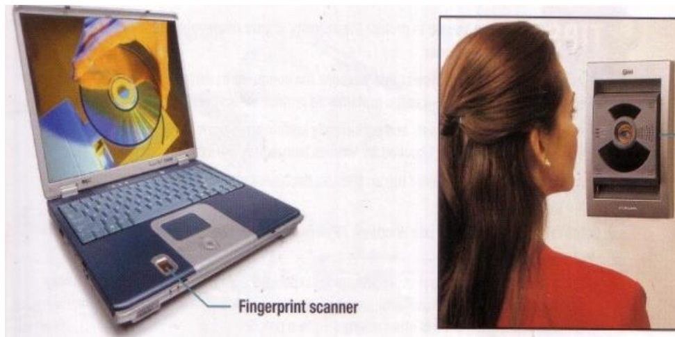
Figure 3.5d biometric devices – Fingerprint scanner (left) & retinal scan (right)
